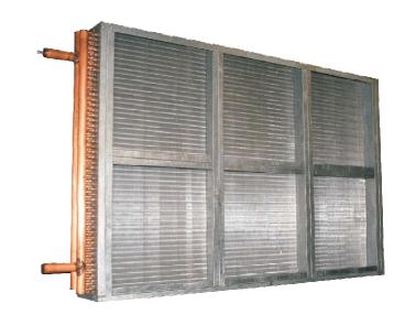
For the usual application of heat transfer, coils are made of copper headers and tubes, with aluminum fins and galvanized steel frames.
