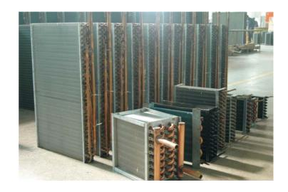
Coil frames are designed to support the finned core, and prevent strains caused by expansion and contraction of finned core. Heavy gauge galvanized steel tube sheets are provided with drawn collars to prevent wearing and chafing of tubes.
